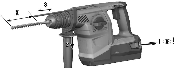
1. Press the release button on the side handle.
