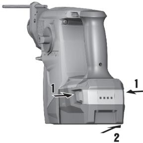
1. Press the release buttons on the battery.
