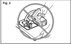
Never attempt to saw with the circular saw held upside down in a vise. This is extremely dangerous and can lead to serious accidents.
